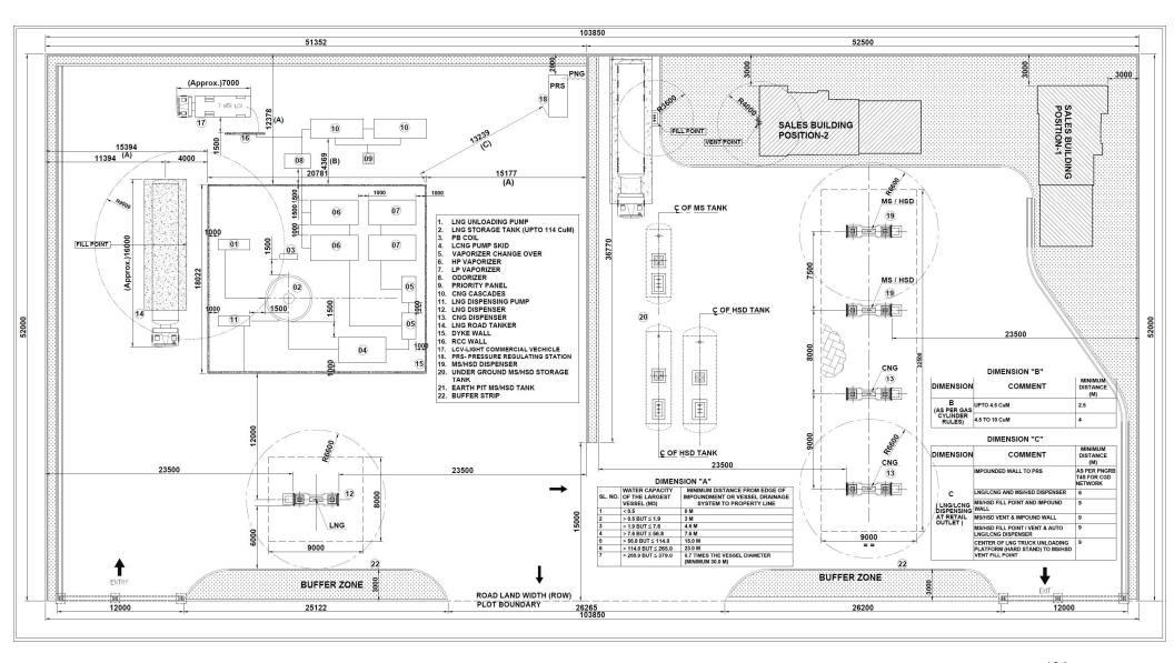
Layout – II. Typical layout of Auto LNG / LCNG dispensing Station co-located with Petroleum (MS, HSD) Retail outlet
